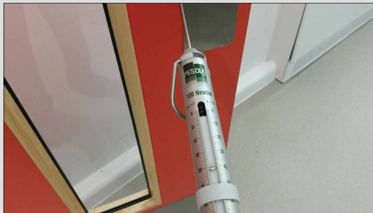
Using a Pesola Gauge to measure the opening force of a door.
