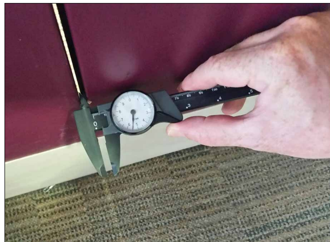
Checking a double door meeting gap with dial calipers during a Type 2 inspection.
